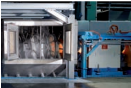
The full-annealed pipes are cooled to 900 °C at high water pressure. Top: Temperature control at the interface to the water cooling.
