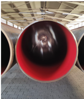
Flow Coat on the pipe interior
