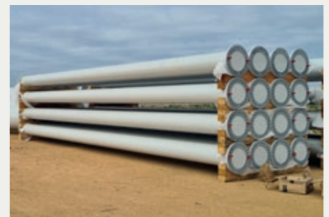
Above: The HFI-welded tubes manufactured in Hamm and Siegen were further processed in Spain before being shipped to Morocco.
