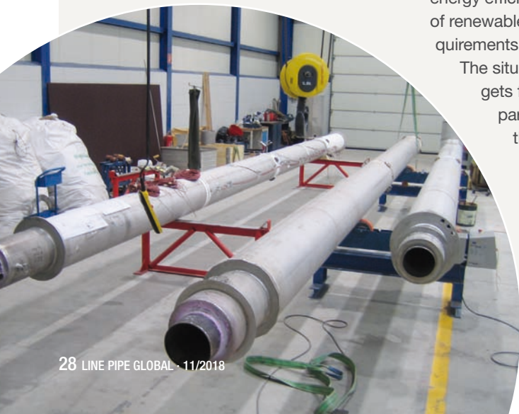
The newly developed HFI-welded steel tubes of grade X8Ni9 may be put to future use in the renewables sector.
